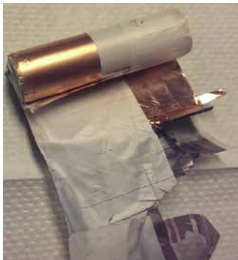
Figure 2: Cell being dissected to study tabs and electrodes designs
